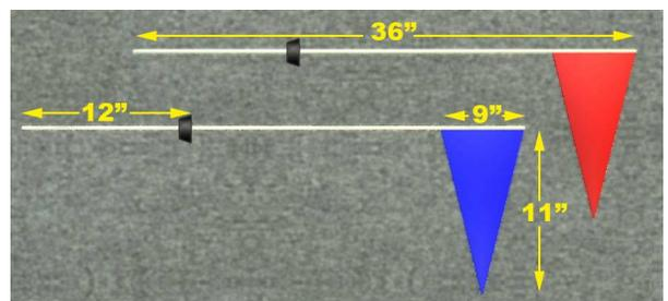
LAP INDICATOR – A FIRST-provided device that is used to automatically record each time the ROBOT CROSSES the FINISH LINE. The LAP INDICATOR is provided to teams at each official competition event. The LAP INDICATOR is attached to the flag pole and must be mounted on the ROBOT as specified in Rule <R18>.
