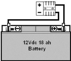
The diagram shows a rectangular battery labeled "12Vdc 18 ah Battery". Two Anderson-style cable connectors are attached to the top of the battery. One connector is connected to the positive terminal, and the other is connected to the negative terminal. The cables extend upwards from the battery.
