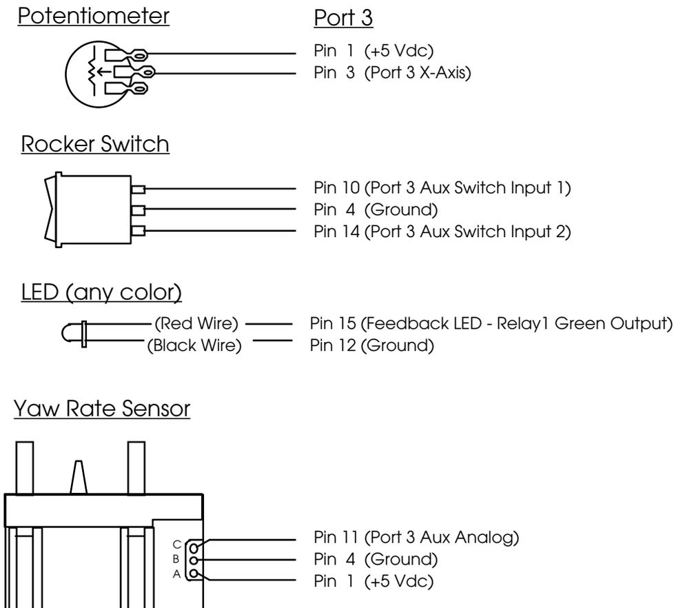
Figure 2.5: Connection Examples for Operator Interface
