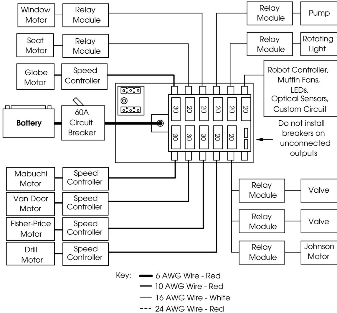
**Figure 2.1: +12 Vdc power distribution**
