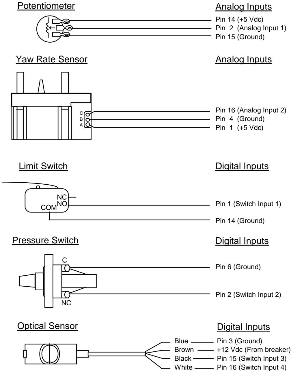
**Figure 2.4: Connection Examples for Robot Controller**
