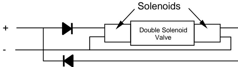
Figure 2.3: Use of Diodes with Double Solenoid Valve
