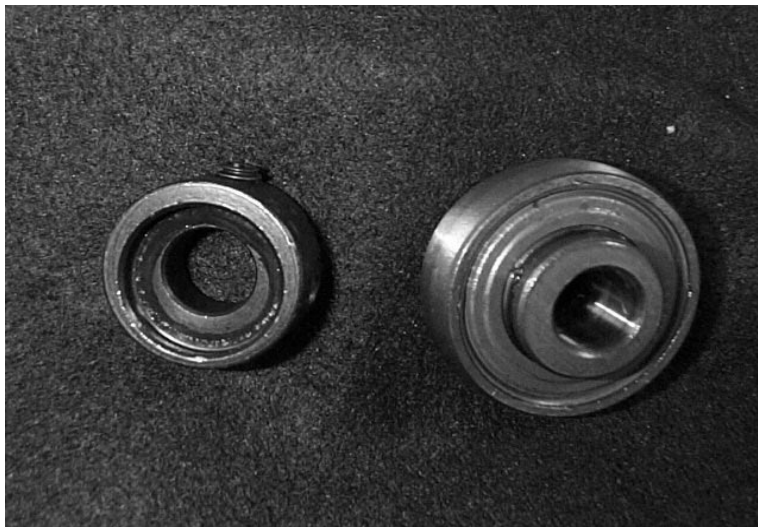
Picture 2 : Self -locking Collar, Radial Ball Bearing with Spherical O.D., ½ in. I.D. (4)
