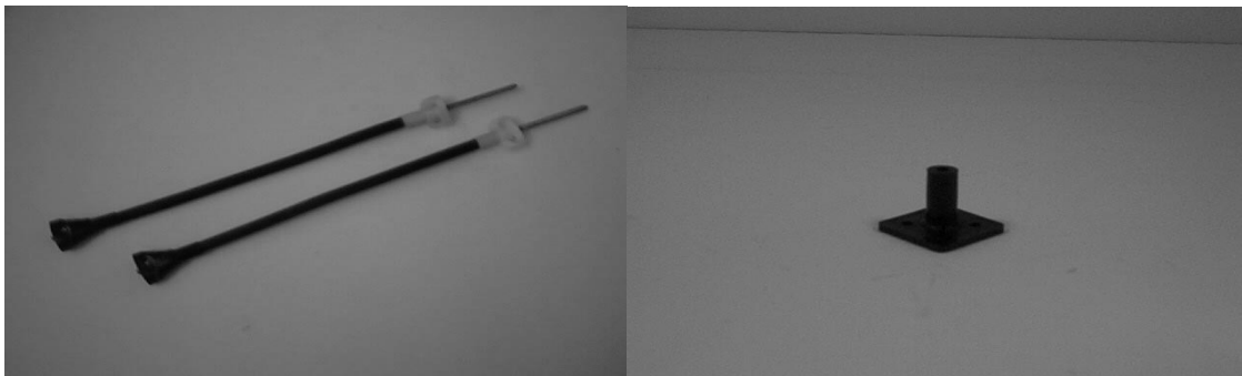
Picture 2: Flexible Motor Shaft (2), Flexible Shaft Coupling (2)
